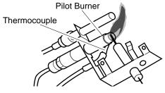
Figure 26 - Incorrect Pilot Flame Pattern
